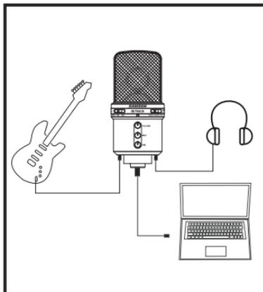
1. Set the G Track up on the included desk stand or any standard mic stand and ensure it is secure and stable. Since the microphone is unidirectional, be sure to face the front side, with the G Track logo, towards the vocalist.
